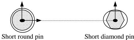
**Figure 4.8.** Locating points for pin-hole locating.
