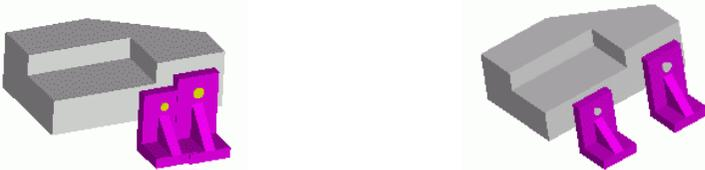
(a) Distance changed between interfering parts to avoid interference
