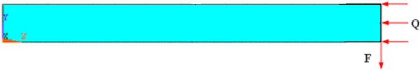
Figure 5.25. An equivalent single continuous beam.
